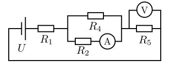
b) The voltmeter reading is simply the voltage on  $R_5$  and so is  $I_{\text{tot}}R_5 = 4.5 \text{ V}$  (2 points).
