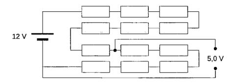
12 similar resistors in series, the voltage drops an equal amount in every resistor. Therefore the voltage across 5 resistors is 5 V.
