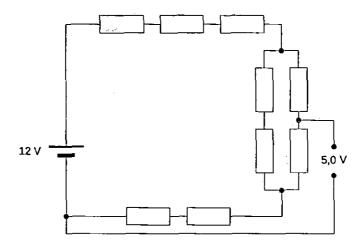
Let's think first 6 equal resistors in series, for every resistor there is a 2 V drop. One of the resistors is replaced with a circuit of 2 in serial, 2 in parallel resistors, like in d). Output for is 5 V is taken as shown in the picture.
