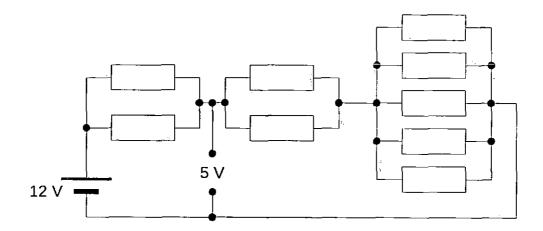
Total resistance is (5+5+2)  $\Omega=12$   $\Omega$ , thus the output shown the has 5 V voltage. Total current is  $I=\frac{U}{R}=\frac{12\,V}{12\,\Omega}=1,0\,A$ . For example in the two leftmost parallel resistors the current is divided in two, and the power of each resistor is  $P=RI^2=10\,\Omega\cdot(0,5\,A)^2=2,5\,W$ . This is over the 1 W specification, and the circuit may fail.
