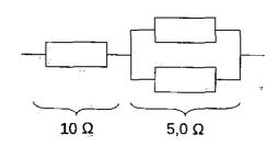
$$R_{tot} = 10 \Omega + 1 / \left( \frac{2}{10 \Omega} \right) = 15 \Omega$$
